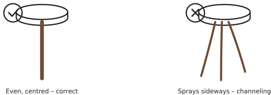
Fig. 5: Correct extraction (left) and channeling (right)
